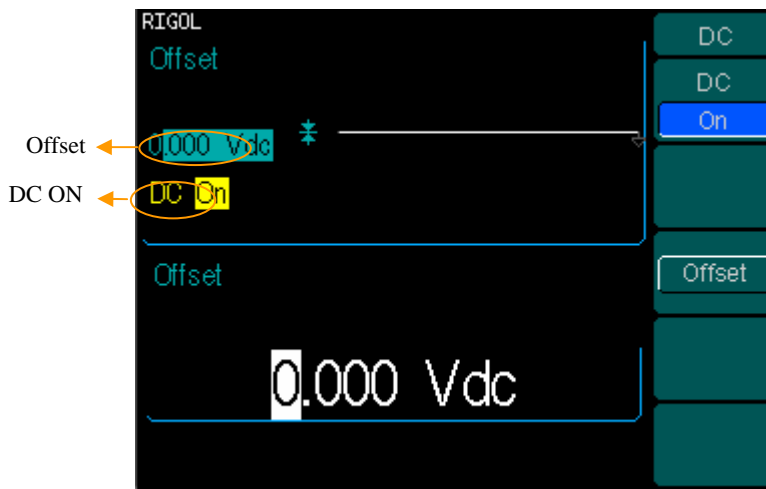
Figure 2—62 DC Setting Interface
